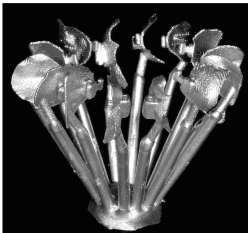
Figure 6. Investment cast lingual brackets after shell removal.
